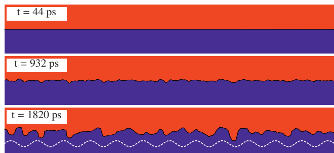
Fig. 1. Time series of images from a g = 1.3 \times 10^{10} g_{Earth} simulation of the RTI. Red is the heavy fluid; blue is the light fluid. Dashed line: reference sine curve corresponding to the predicted wavenumber of maximum instability k_m .
